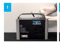
Add one bottle of 100 ml Power-Clean AC Bacteria & Odour Remover in to the machine.
