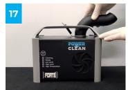
Remove outlet tube and dispose of residue.
