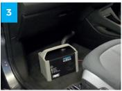
Place the machine upright, in a level position in the front passenger footwell.
