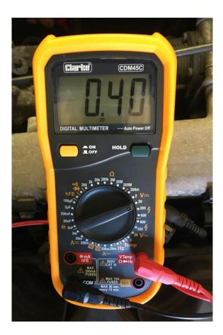
Multimeter on the signal wire KOEO (Key on engine off) should be no more than 0.5v. If higher than 0.7v sensor replacement recommended.
