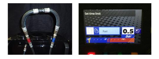
The blue pressure bar should not increase above 0.7 bar. You may see the unregulated pressure banner flashing on the screen - this is normal.
