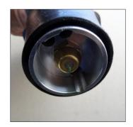
Prolonged contact with the Intake product can cause the rubber cone to swell.
