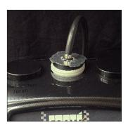
NOTE: do not leave fluid in the tank with the atomiser sat in the tank opening. Evaporation of the product will cause the rubber cone to swell.
